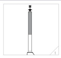
Drive the aluminium insert out of the steerer tube.(fig. 1)
