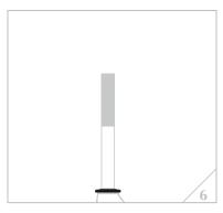
• Knock the fork cone onto its seat on the steerer tube using an appropriate mounting tube.
