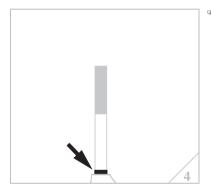
Slightly grease the bearing surface for the fork cone.
