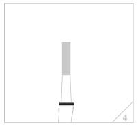
Fit the lower bearing of your headset onto the steerer tube without using any lubricant or grease. Be careful to orient the lower bearing correctly.
