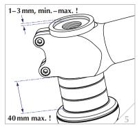
Assemble the fork, spacer, stem and headset in the head tube of your bike frame in accordance with the manufacturer's instructions.
