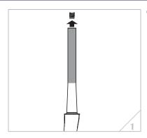
Unscrew the aluminium insert from the steerer tube.(fig. 1)
